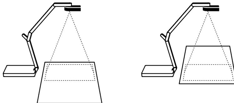
Text document in one position under Ziggi-HD with camera lens capturing top half of document, then moved "up" so that the camera lens is capturing the bottom half of document
