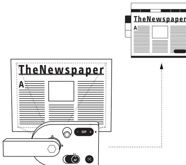
The top of the Ziggi camera lens is located 90° counterclockwise from the square top of the camera body
